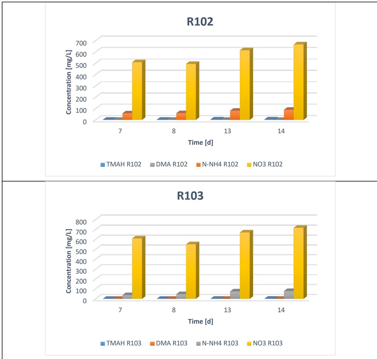
Figure 3.2: Concentration of TMAH, DMA, N-NH<sub>4</sub><sup>+</sup> and NO<sub>3</sub><sup>-</sup> for R101, R102 and R103 during the period 12/06/18 – 19/06/18 (batch operation)
