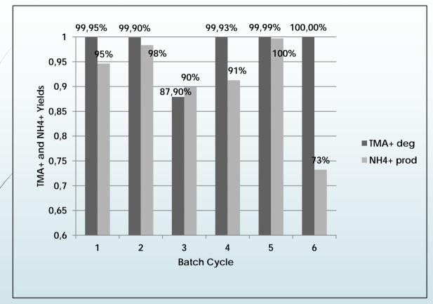
The experiments on wastewater have showed that biological treatment is able to remove TMAH with and efficiency greater than 99%, as TMAH removal yield, after about 6 days of process.
